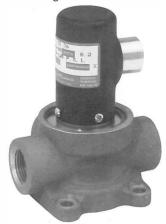
590E1 590E1-3-10-36 Model 590E1 is a single-solenoid, maintained-contact, spring-return, 2-way or 3-way valve available either normally closed or normally open.
