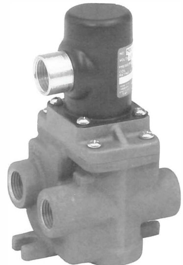
501-4E1 501-4E1 Model 501-4E1 is a single-solenoid, maintained-contact, spring-return, 4-way, 4-port valve with common inlet and common exhaust. Cylinder port #1 is normally open; cylinder port #2 is normally closed.
