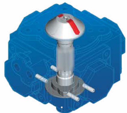
Limit stop for open-close and intermediate positions
