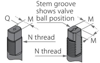
Stem groove shows valve ball position
