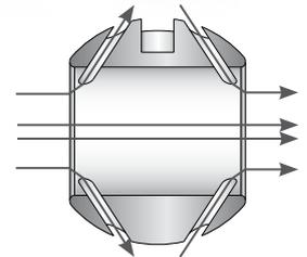
With the valve in the open position, special tunnels flush the valve cavity constantly
