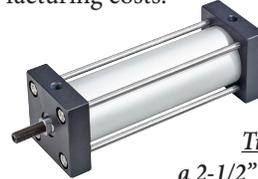
*Tie-rod construction shown on a 2-1/2" bore x 7" stroke cylinder with male rod extension. (Model S521-7-MR)*
